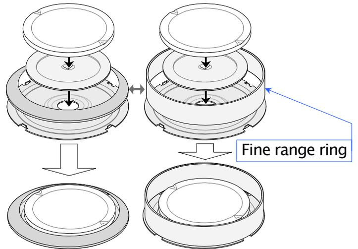
Use the fine range ring to avoid errors caused by drafts when weighing with a minimum display of 0.01 mg.
