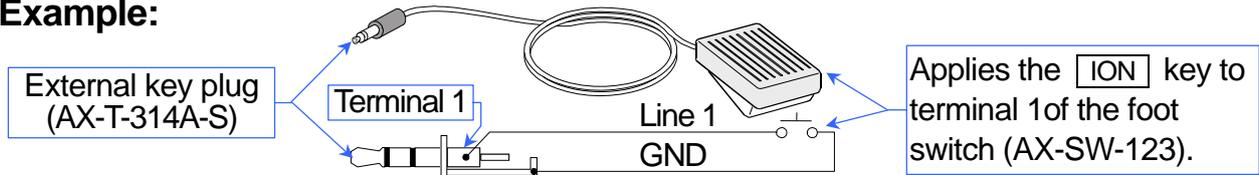
Applies the **ION** key to terminal 1 of the foot switch (AX-SW-123).
