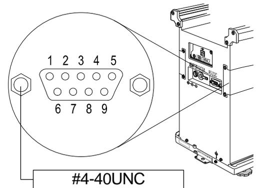
Signal names of the balance side are the same as the DTE side with TXD and RXD reversed.
